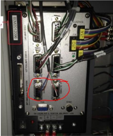
Newer machines will look like this. Find the Cable labeled "COM2" and disconnect and reconnect the cable. In this case it is Cable B.
