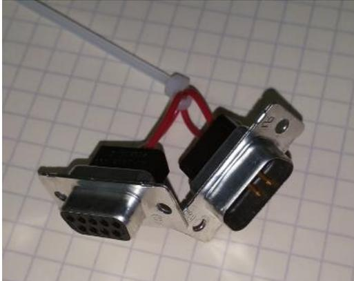
These may be provided to you, either included in the PypeServer kiosk enclosure, or sent to you. Or you can create your own. Here are the back sides of the connectors. The male connector on left, female connector on right.
